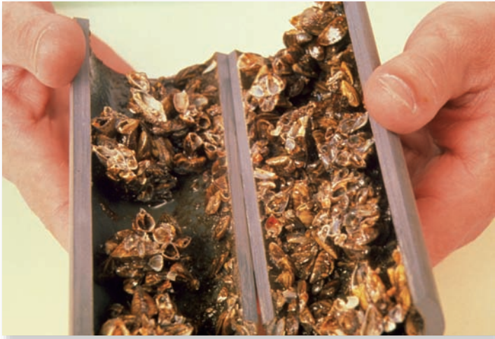
Figure 60.16 Zebra mussels ( Dreissena polymorpha ) clogging a pipe. These mussels were introduced from Europe, and are now a major problem in North American rivers.
